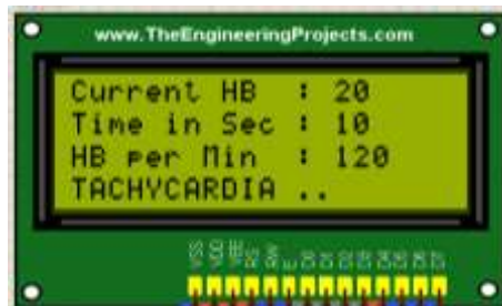
Fig. 6. The result of Heart Rate simulation
